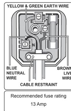
Double insulated products, which are always marked with this symbol
